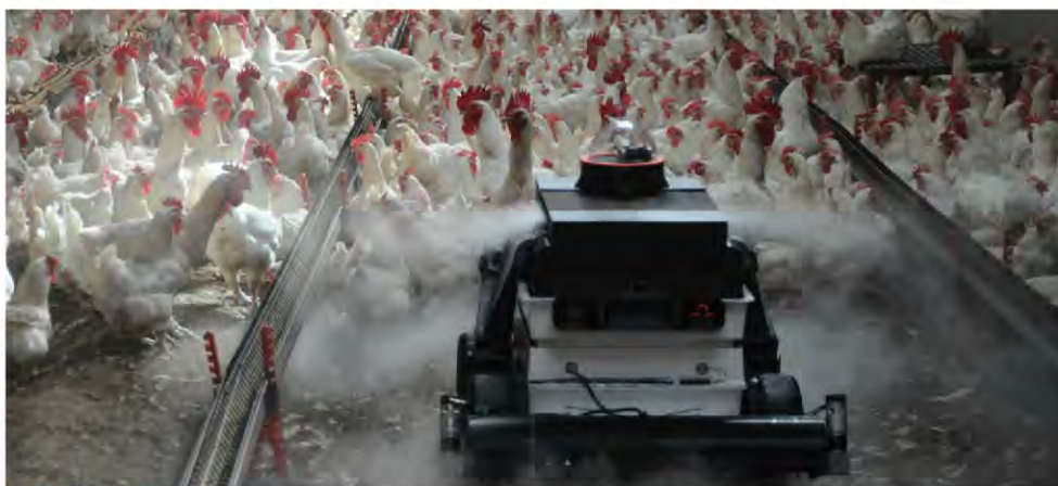
OCTOPUS ROBOTS | Able to turn and aerate poultry bedding, with the minimum disturbance to birds
